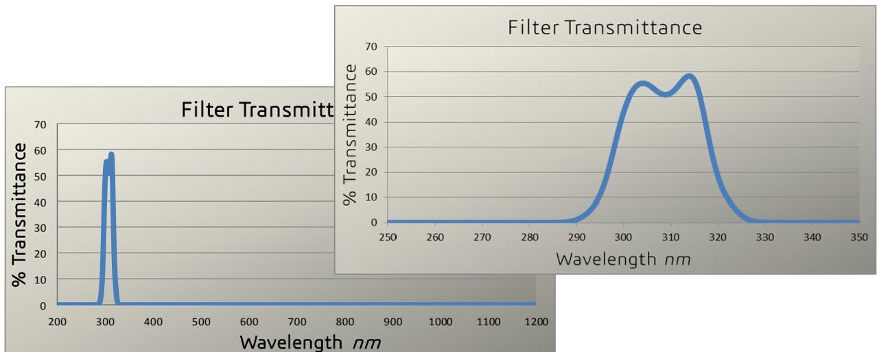
CWL 308nm  $\pm$  2.5nm, FWHM 20nm  $\pm$  2nm, Peak Transmission 40% min., Blocking UV to 1200nm OD > 4
