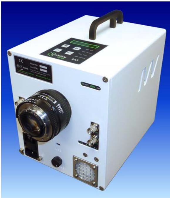
Available with both S20 and S25 photo-cathodes, the unique patented system offers deep UV to visible response (**200 to 900nm**) with modest system gain into a P46 (green) fast decay output phosphor, but may also be coupled to a front end MCP derived intensifier (reducing linearity & MTF/resolution) for higher gain or faster gating.
